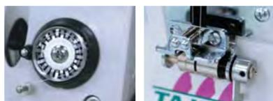
Thread breakage detector Middle thread guide with thread take-up spring
